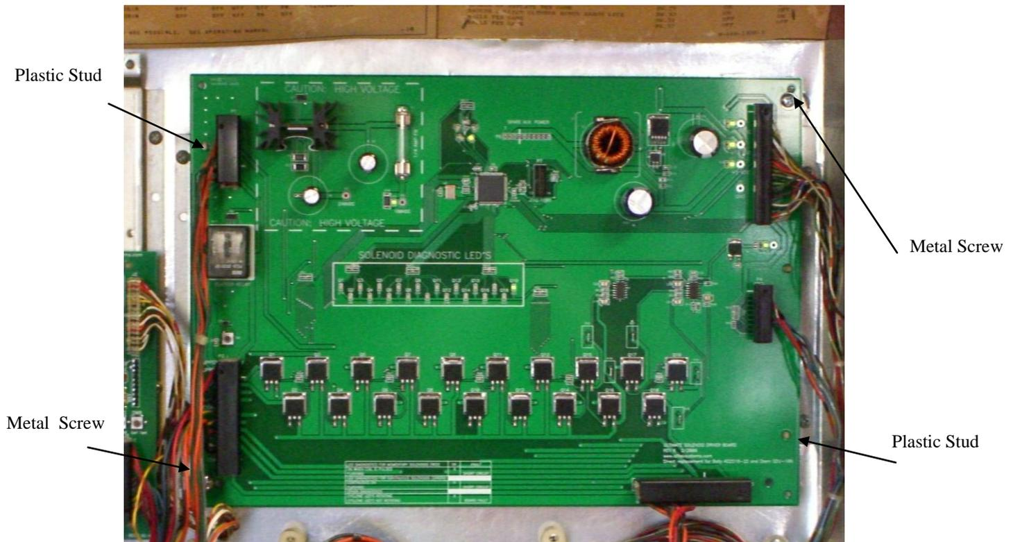
Now let's talk about safety issues. If you look at the SDB you will notice a section labeled High Voltage in the upper left corner. The games use a high voltage power supply to power the displays. NEVER put your hands in this area when power is applied. Allow time for capacitors to discharge before handling the board. If in doubt please contact customer service.
